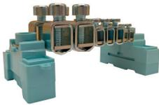
**Branching terminal boards** are designed for multiple branching, multiple adaptors or mutual connection of conductors with various cross-sections (from 2,5 mm<sup>2</sup> to 95 mm<sup>2</sup> for terminal board series 2; from 1,5 mm<sup>2</sup> to 16 mm<sup>2</sup> for terminal board series 3). The connecting and branching part of the terminal board consists of a connecting brass bridge (galvanised) and steel fastening clamps (galvanised).
