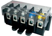
**DTS distribution blocks** are used for the connection of four- and five-conductors cables in electric installations. They provide power distribution in various applications. They are offered in versions for all types of Al and Cu conductors from 1,5 to 150 mm<sup>2</sup>. The blocks can be attached on the plate or on the DIN rail TH using a holder. Material: casing - PA6 polyamide, V0, cover – transparent polycarbonate – PC. Operating temperature -25 ÷ + 100°C.
